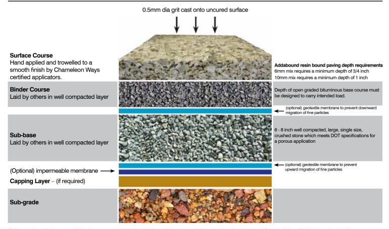
Sub-grade, sub-base and binder courses must be designed by an engineer as depth and type of materials will change depending on intending load.
